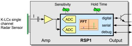
Fig. 3: Typical single channel architecture
