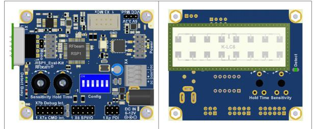
RSP1\_Eval-Kit; Left: K-LC2 sensor on front connector; Right: Backside equipped with K-LC6 sensor
