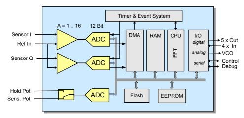
Fig. 4: RSP1 simplified block diagram
