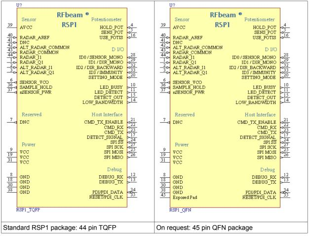
Fig. 13: RSP1 Pin Configuration: left TQFP case, right QFN case
