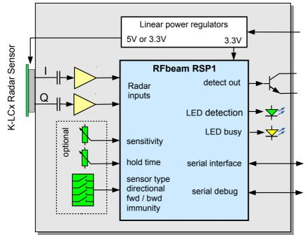
Fig. 1: Typical stand-alone application circuitry
