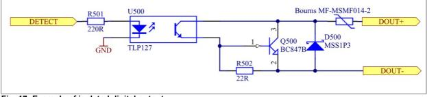
Fig. 17: Example of isolated digital output
