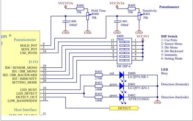
Fig. 16: Stand alone configuration, control elements
