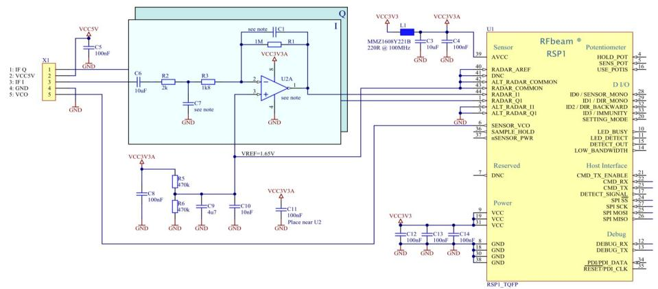
Fig. 14: Single Amp example for K-LCx sensors. Channel Q circuit is equivalent to channel I
