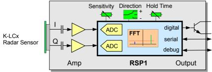
Fig. 2: Typical dual channel architecture
